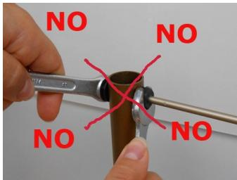
Insert elements as shown in the figure, hand tighten the nut M8 Nylon (**do not use keys as the material used has a self - locking function**)
