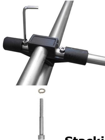
Match the dipoles with M4x35 mm and washer as shown in photo, secure the half dipoles of 12 mm Ø by using the Allen Key of 3mm and the collar for the fixing of the Bazooka.
