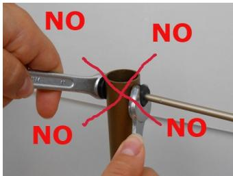
Insert elements as shown in the figure, hand tighten the nut M8 Nylon (**do not use keys as the material used has a self – locking function**)
