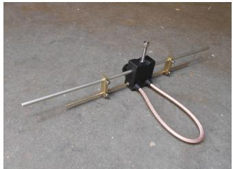
Match the dipole with M5x35 mm and washer as shown in photo
