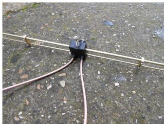
Match the dipoles with M5x35 mm and washer as shown in photo
