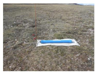
The **ULF30JXX** induction coil is provided with an internal preamplifier and filters which are remotely programmable. Exceptionally low noise, en = 3.5 nV/÷Hz, at 10 Hz, a low 1/f noise corner frequency of 2.7 Hz, and high gain allow accurate high-gain amplification of low-level signals. A gain-bandwidth product of 8 MHz and a 2.8 V/msec slew rate provides excellent dynamic accuracy in high-speed, data acquisition systems.
